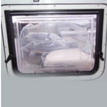
Wind out window with flywire above bench
