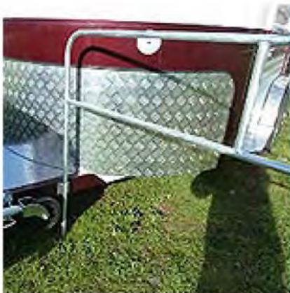
Fencing attachments to rear & front of float
