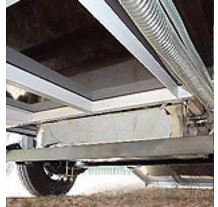
Underfloor 90 litre water tank
