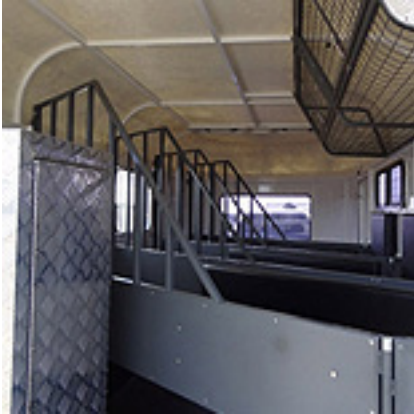
4 Horse float interior - saddle box, stalls & racks
