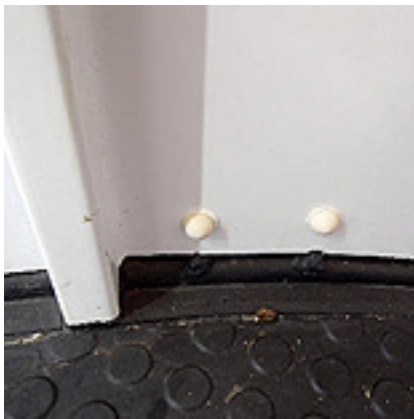
All rivets are rubber backed
